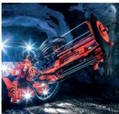
The DL431 electro-hydraulic drill rig is specially designed for production and long-hole drilling in underground mines.
