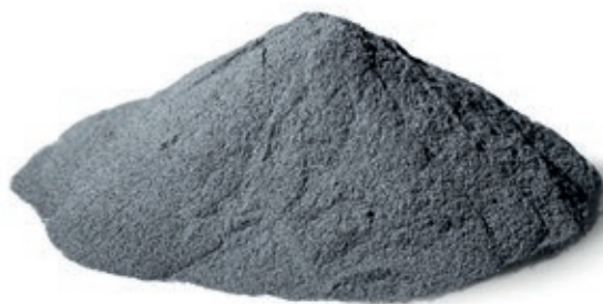
METALLIC POWDER USED FOR MANUFACTURING HIP COMPONENTS
