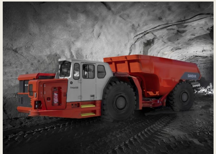
The battery-electric truck Sandvik® TH665B was successfully tested in Australia.
