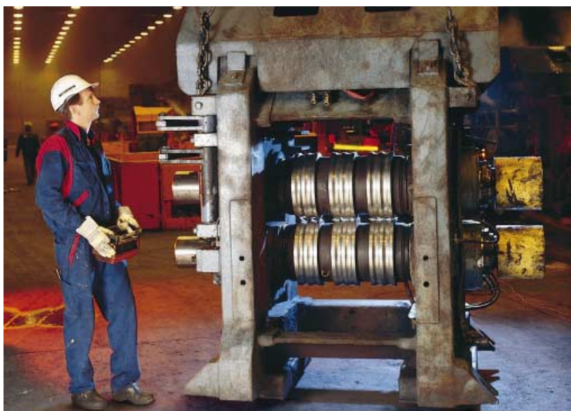
Cast-in-carbide integral rolls, so-called CIC rolls, are a further development of an older technology and are used with great success in the steel industry, among other application areas.
