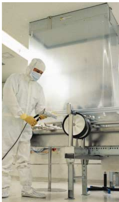
Electro-polished tube for the electronics industry is manufactured at Sandvik Calamo. Tube production is carried out at an extremely high level of cleanliness.
