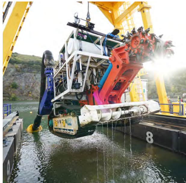
Sandvik supplied a 150 kilowatt hydraulic-driven cutter head, ideal for cutting solid rocks, to an underwater mining project.
