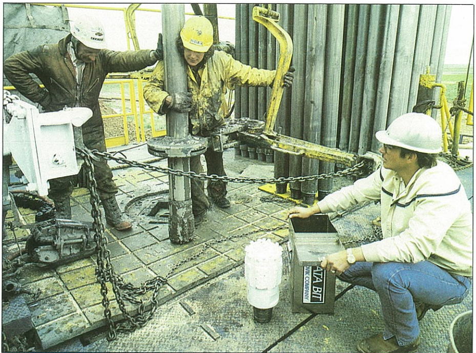
Drill bits for the oil and gas industry are among the new fields that Sandvik Rock Tools has moved into. Our American subsidiary company Strata Bit has developed a special bit armed with industrial diamonds.
