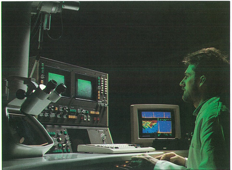
Sandvik's Steel Research Centre in Sandviken has a new transmission electron microscope that can magnify up to 850,000 diameters and is augmented with up-to-date facilities for chemical analysis.
