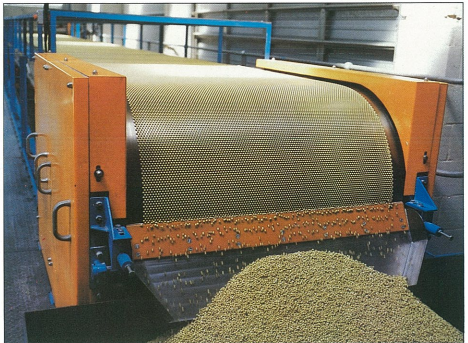
The fine results achieved by Sandvik Process Systems in 1985 were largely due to increased deliveries of Rotoform installations. This picture shows a plant for cooling and pelletizing wax, which the company supplied to a customer in Britain.
