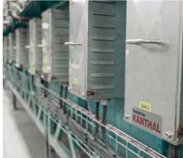
The electric furnace at the Glassit facility requires 37 percent less energy and emits no CO 2 .
